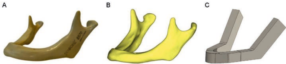
Figure 1. 3D computer modelling of the mandible: (A) Synbone® mandible, (B) DICOM file from CBCT, and (C) a simplified 3D model of a mandible.
