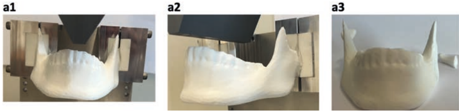
Appendix 1 Figure A4. The break pattern of non-fractured mandible replicas at the maximum failure load. (a) all the mandibles broke at the left fixture side (a1-a3).
