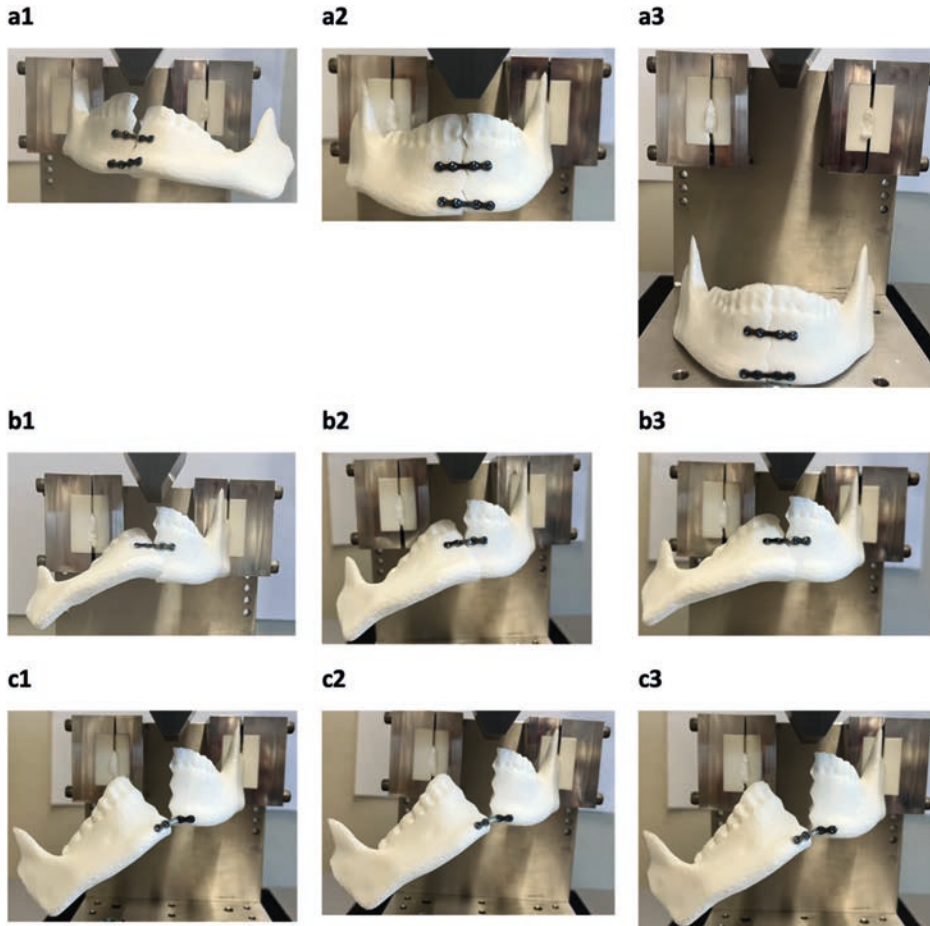
Appendix 1 Figure A1. Breakage pattern of the mandibular symphysis fracture fixed with three different plate configurations at the maximum failure load. $
