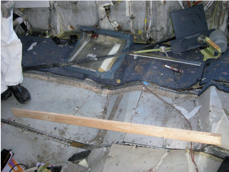
Figure 5. The floor in the front part of the airplane was pushed up.
